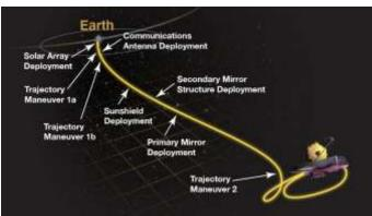
A heat shield keeps the telescope very cold at less than 50 K while solar power panels, radio antenna and the jets are on the hot side at 85oC. The telescope should settle into its halo orbit around the end of January.
