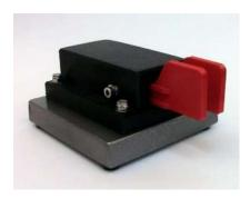
Kenwood TS-830 and other rigs of this generation with valve finals (1970s and 80s) use grid block keying. When the key is open, you can measure -65 volts across the key points.
